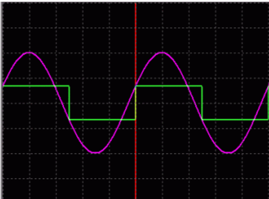
Figure 1b. The same sine wave sampled exactly twice per period generates a square wave—amplitude information is lost.
